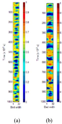
Fig. 8: Images from the ECT sensors stacked in time for the first-10 s of the flow. Time axis increases from top to bottom. (a) Lower plane: Bubble size is large but less than the bed diameter. (b) Upper plane: Bubble size grows to the size of bed diameter, indicating slugging.
