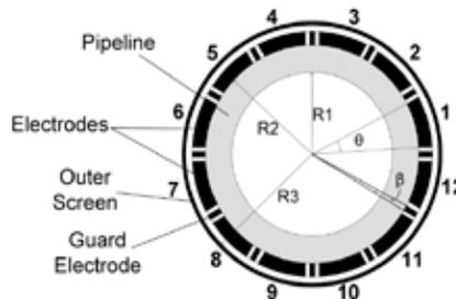
Fig. 1: Structure of an ECT sensor with 12 electrodes. R1 is the inner pipe wall radius, R2 the outer pipe wall radius and R3 the screen wall radius.  $\theta$  is the electrode angular size and  $\beta$  is the gap within which the guard electrode is  $2.5^\circ$  (Zainal-Mokhtar and Mohamad-Saleh, 2013; Mohamad-Saleh, 2001).
