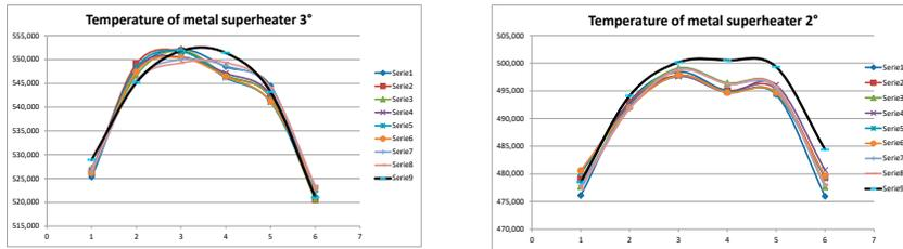
Figure 3.12. Distribution of temperature of superheater metal during testing
