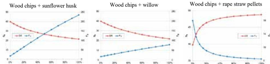
Figure 3.3. Changes in value of fouling and slagging indexes for a mixture of wood chips with different kinds of biomass with a variable mass share.
