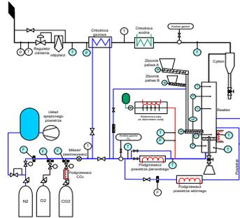
Figure 3.5. Flow diagram of experimental installation with BFB reactor
