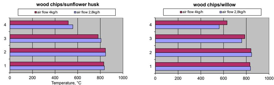
Figure 3.9. Temperature distribution along the height of the reactor during the combustion of the mixture with sunflower husk
