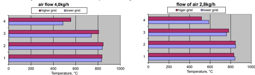
Figure 3.8. Temperature distribution along the height of the reactor, depending on the grain size
