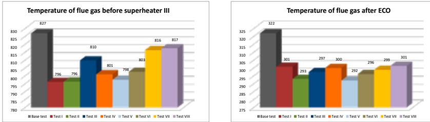
Figure 3.11. The flue gas temperature for different surfaces during the verification tests
