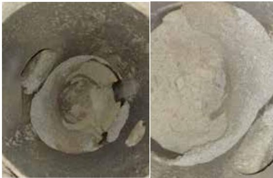
Figure 3.6. View of the reactor interior and sinter of bed material
