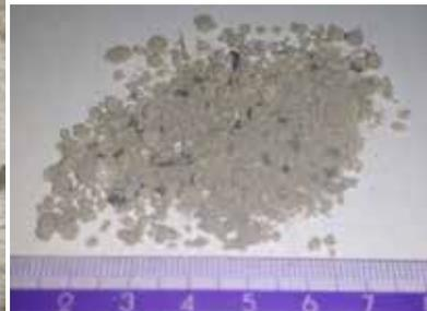
Figure 3.7. Bed material after combustion of fuel mix : sunflower husk and wood chips
