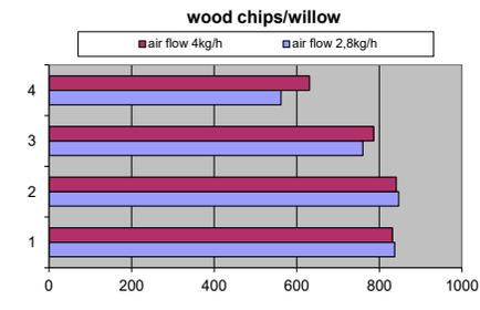
Figure 3.10. Temperature distribution along the height of the reactor during the combustion of the mixture with willow
