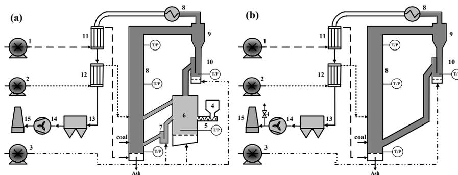
1-primary air fan, 2-secondary air fan, 3-air fan for pyrolyzer, 4-feedstock hopper, 5-screw feeder, 6-FB pyrolyzer, 7-downstream loop seal, 8-TFB combustor, 9-cyclone, 10-upstream loop seal, 11- primary air heat exchanger, 12-secondary air heat exchanger, 13-bag-type dust collector, 14-induced fan, 15-chimney
