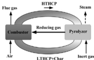
Fig.1. Basic principle of decoupling combustion process.
