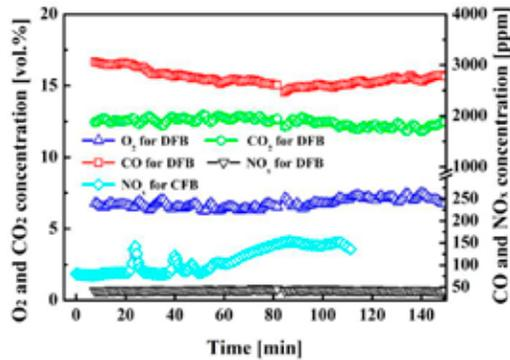
Fig. 6. Comparison of gas components in flue gas for DFB and CFB system
