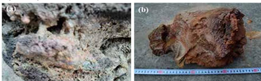
Fig. 5. Picture of slag in the combustor (a) and loop seal (b) for the CFB system
