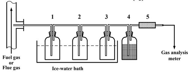
1/2/3 Ice-water bath, 4-silica gel drying bottle,5-filter
