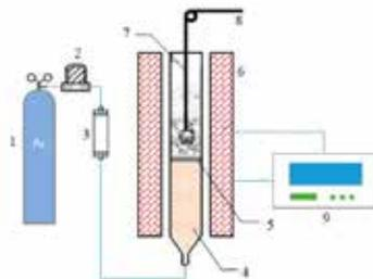
Fig. 1. Schematic diagram of the experimental setup: 1. Argon gas cylinder; 2. Gas control valve; 3. Float flowmeter; 4. Quartz glass preheating section; 5. Distributor; 6. Electric heating furnace; 7. Hanging basket; 8. Feeding pulley; 9. Thermoelectric thermometer
