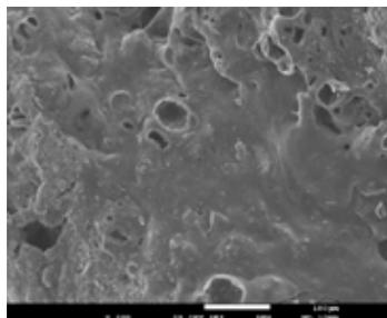
Fig. 4. External structure of char particle(Group C,  $d_p=719.20\mu\text{m}$ ,  $T=800^\circ\text{C}$ )
