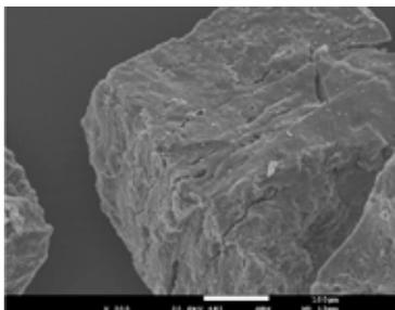
Fig. 3. External structure of char particle(Group A,  $d_p=177.03\mu\text{m}$ ,  $T=800^\circ\text{C}$ )
