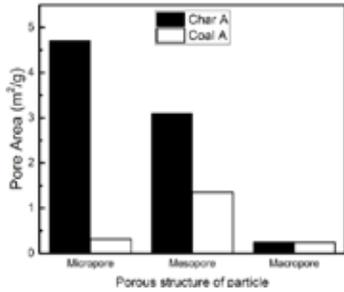
Fig. 8. Comparison of porous structures between coal and char of Group A
