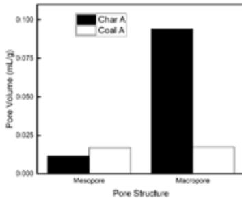
Fig. 10. Comparison of porous structures between coal and char of Group A
