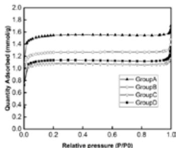
Fig. 7. Adsorption isotherm of char particles at the pyrolysis temperature of 800 °C
