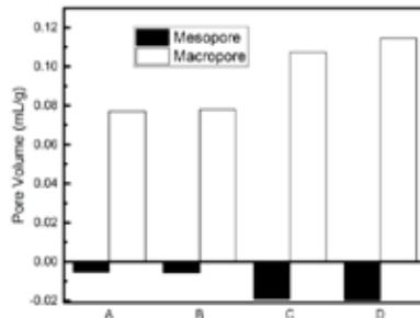
Fig. 11. Change of porous structure after pyrolysis for each group.
