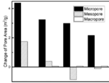
Fig. 9. Change of porous structure after pyrolysis for each group.
