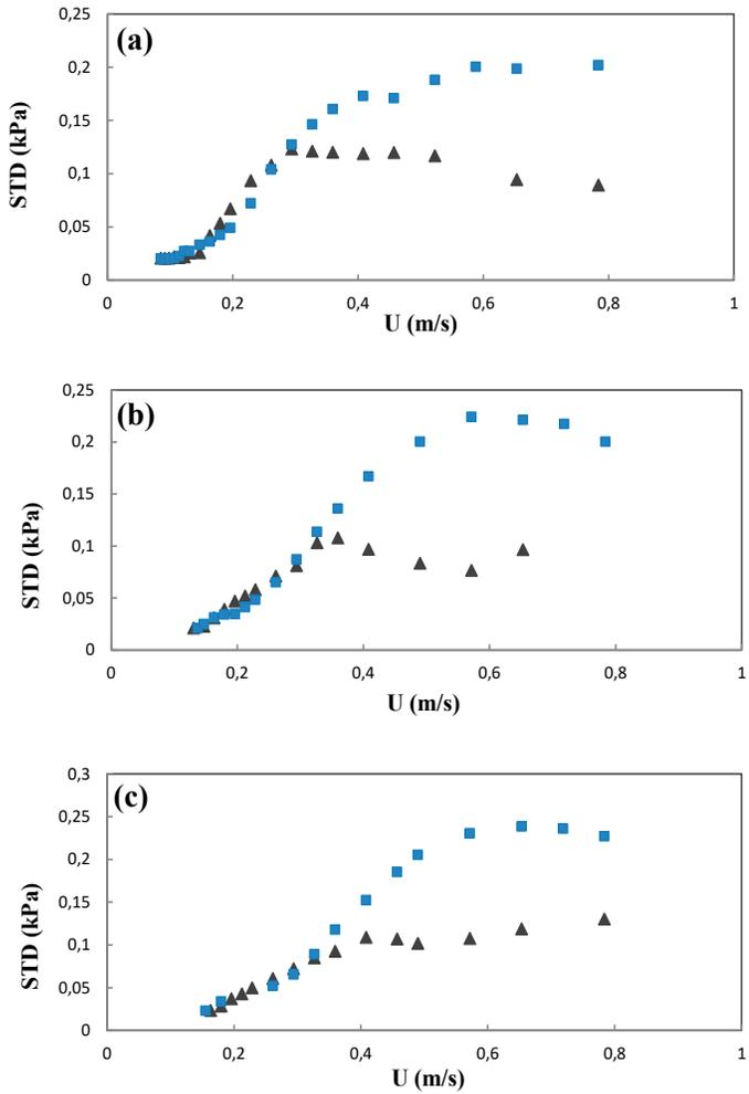
Fig. 4. Standard deviation of pressure fluctuations as a function of superficial gas velocity, (a)  $d_p=0.275$  mm, (b)  $d_p=0.460$  mm, (c)  $d_p=0.600$  mm: charged particles ( $\blacktriangle$ ) and uncharged particles ( $\blacksquare$ )
