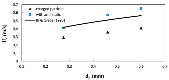
Fig. 5. Calculated and experimental transition velocities to for beds of charged particles and the bed containing anti-static agent.
