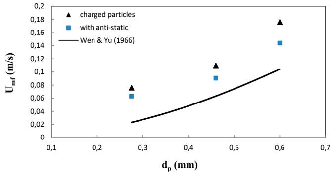
Fig. 3. Calculated and experimental minimum fluidization velocities for beds of charged particles and the bed containing anti-static agent.
