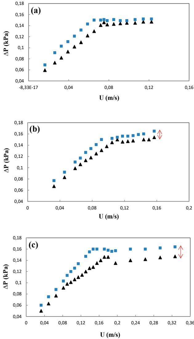
Fig. 2. Pressure drop as a function of gas velocity in beds of various particle size, (a)  $d_p=0.275$  mm, (b)  $d_p=0.460$  mm, (c)  $d_p=0.600$  mm: charged particles (▲) and uncharged particles (■)
