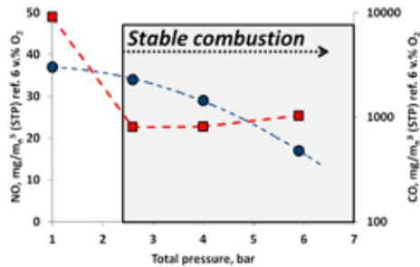
Fig. 2. The comparison of NO and CO emissions during combustion of "Ziemowit" hard coal (circles NO, squares CO)
