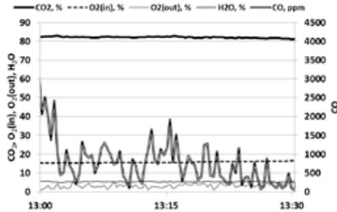
Fig. 1. Measured composition of flue gas during combustion of "Ziemowit" hard coal under pressure of 4 bar
