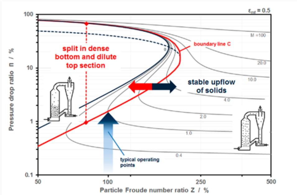
Fig. 3: Flow behavior of ash in the combustion chamber of CFB in the Enefit280 process; Model: Steady-state model for heterogeneous fluid-solid flow according to Wirth (1990)
