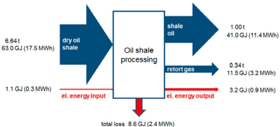
Fig. 4: Specific energy balance of the Enefit280 process for the production of 1.0 ton of shale oil; the width of the arrows represents the energy content of the individual process streams
