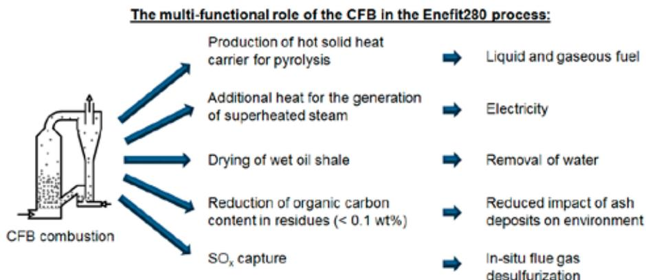
Fig. 2: The multi-functional role of the CFB combustion unit in the Enefit280 process
