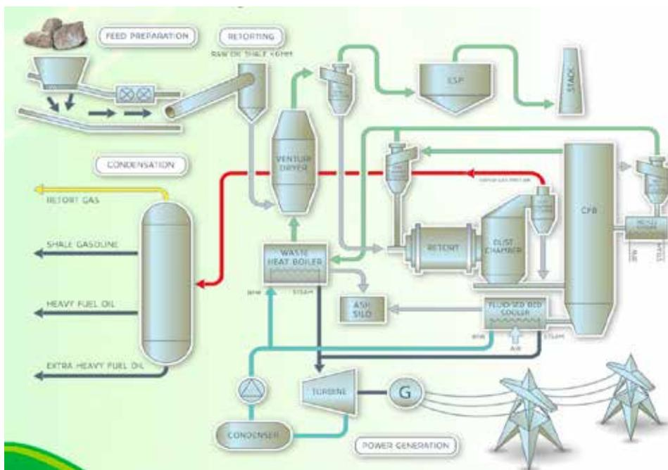
Fig. 1: Schematic representation of the process flows and unit operations in the Enefit280 process
