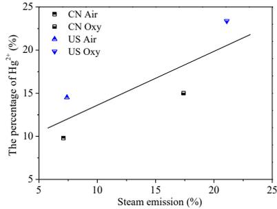
Fig. 8. Effect of steam emission on mercury oxidation under air and O<sub>2</sub>/CO<sub>2</sub> atmosphere with different coals.
