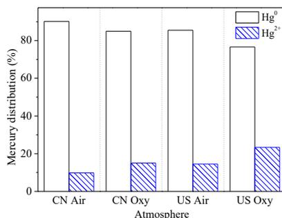
Fig. 4. Mercury emission and its speciation under air and  $O_2/CO_2$  atmosphere with different coals.
