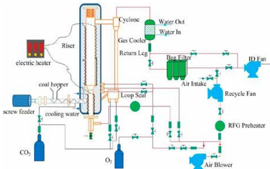
Fig. 1. Schematic diagram of mercury oxidation during warm recycle oxy-coal atmosphere in circulating fluidized bed.
