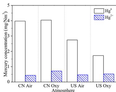
Fig. 3. Mercury concentration under air and  $O_2/CO_2$  atmosphere with different coals.
