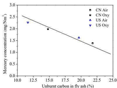
Fig. 5. Effect of unburnt carbon on particulate mercury under air and  $O_2/CO_2$  atmosphere with different coals.
