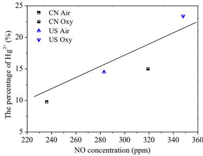
Fig. 7. Effect of NO emission on mercury oxidation under air and O<sub>2</sub>/CO<sub>2</sub> atmosphere with different coals.
