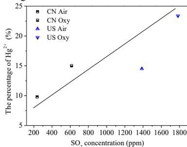
Fig. 9. Effect of SO<sub>2</sub> emission on mercury oxidation under air and O<sub>2</sub>/CO<sub>2</sub> atmosphere with different coals.
