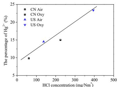
Fig. 6. Effect of HCl emission on mercury concentration under air and  $O_2/CO_2$  atmosphere with different coals.
