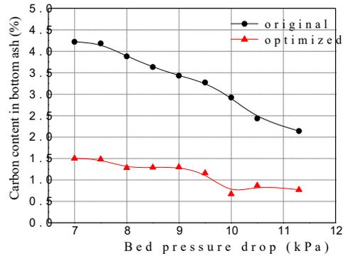
Fig.1 Burnout properties of the four coals Fig.2 The carbon content in bottom ash before and after optimization
