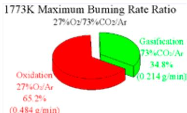
Fig. 8. Meng coal char maximum burning rate ratio for oxidation and gasification in 1773K
