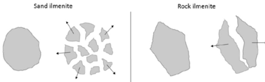
Figure 5 – Schematic sketch of the morphological change and the possible ways for particle degradation of sand and rock ilmenite particles during 15 days of exposure.
