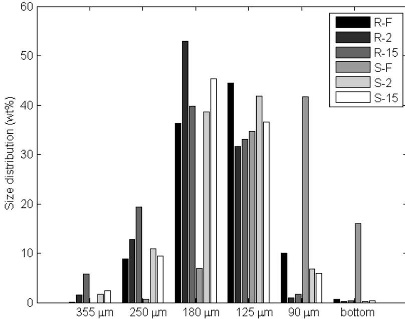
Fig. 3. Sieving curves obtained through sieving of sand and rock ilmenite in as-received condition as well as after 2 and 5 days of exposure. R stands for rock, S for sand, F for fresh material, 2 and 15 are the amount of days that the material has been used as bed material before extraction.
