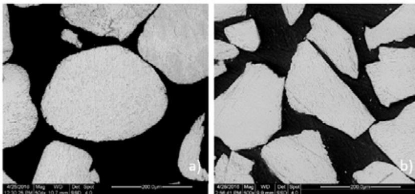
Fig. 1. SEM micrographs of ilmenite particles used as bed material during the experiments: a) sand ilmenite; b) rock ilmenite.
