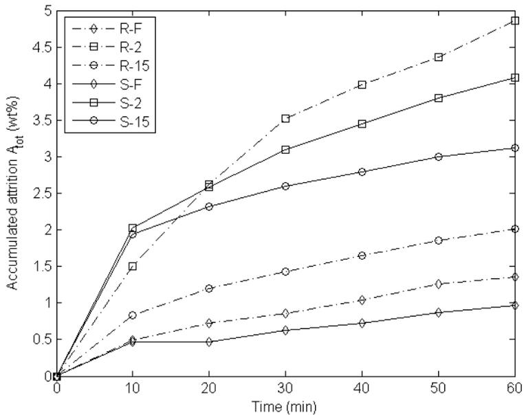
Fig. 4. Accumulated attrition measured on sand, S (solid lines) and rock, R (dashed lines) ilmenite in “as-received” conditions but also after 2 and 15 days of exposure. Diamond markers represent fresh material, F, square and circular markers represent material that has been extracted after 2 and 15 days of operation in the combustor, respectively.
