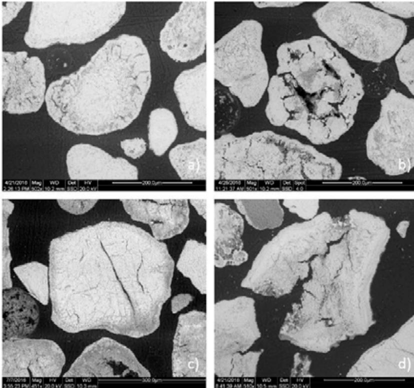
Fig. 2. SEM micrographs of cross-section of ilmenite particles extracted after 2 and 15 days of exposure where a) and b) are sand ilmenite and c) and d) are rock ilmenite.
